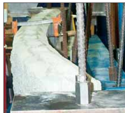
Top bond beam deflection.
