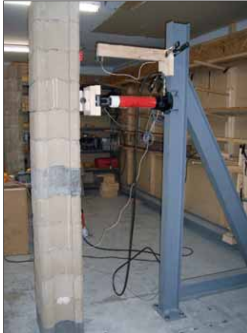
Hydraulic ram and frame assembly for AB Fence Post flexural test.
